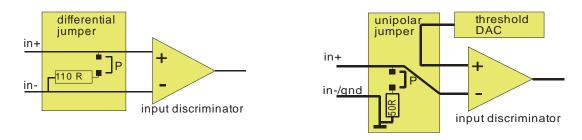
"P" means jumper position near to front panel, then input is terminated.
