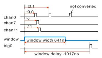
The trig0 -1017 ns is the virtual start for the data. Channel resolution is selected to 1/64 ns (15.6 ps) The generated event structure looks as follows (channels are in arbitrary order):
